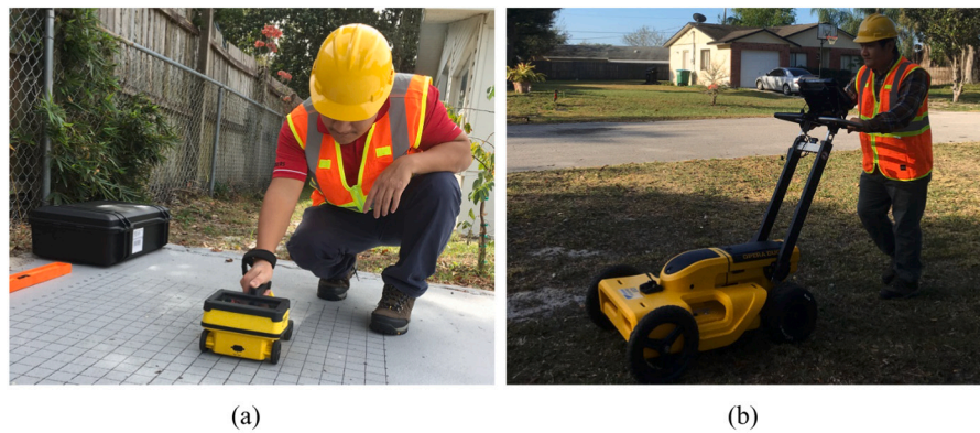
Fig. 1. Commonly-used GPR systems for (a) concrete scanning and (b) utility locating.
