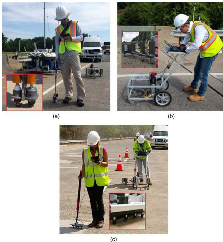
Fig. 1. NDE technologies (images by Jinyoung Kim): (a) impact echo testing; (b) ultrasonic surface wave testing using PSPA; (c) electrical resistivity testing using Resipod probe
