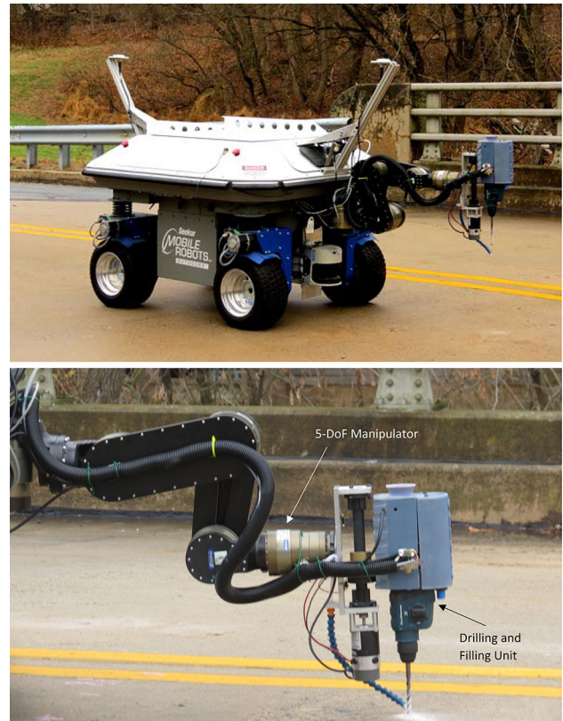
Fig. 14 Mobile manipulator-based autonomous rehabilitation platform ANDERS ( top ), and 5-DoF manipulator with drilling/filling robotic end-effector ( bottom )
