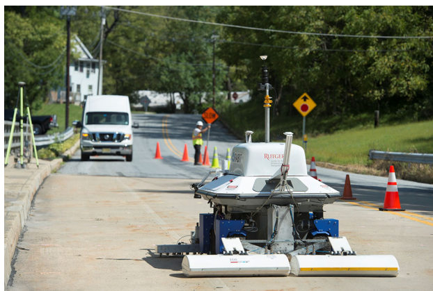
Fig. 7 RABIT data collection on the Pohatcong Creek Bridge (photo: N. Romanenko, Rutgers University)
