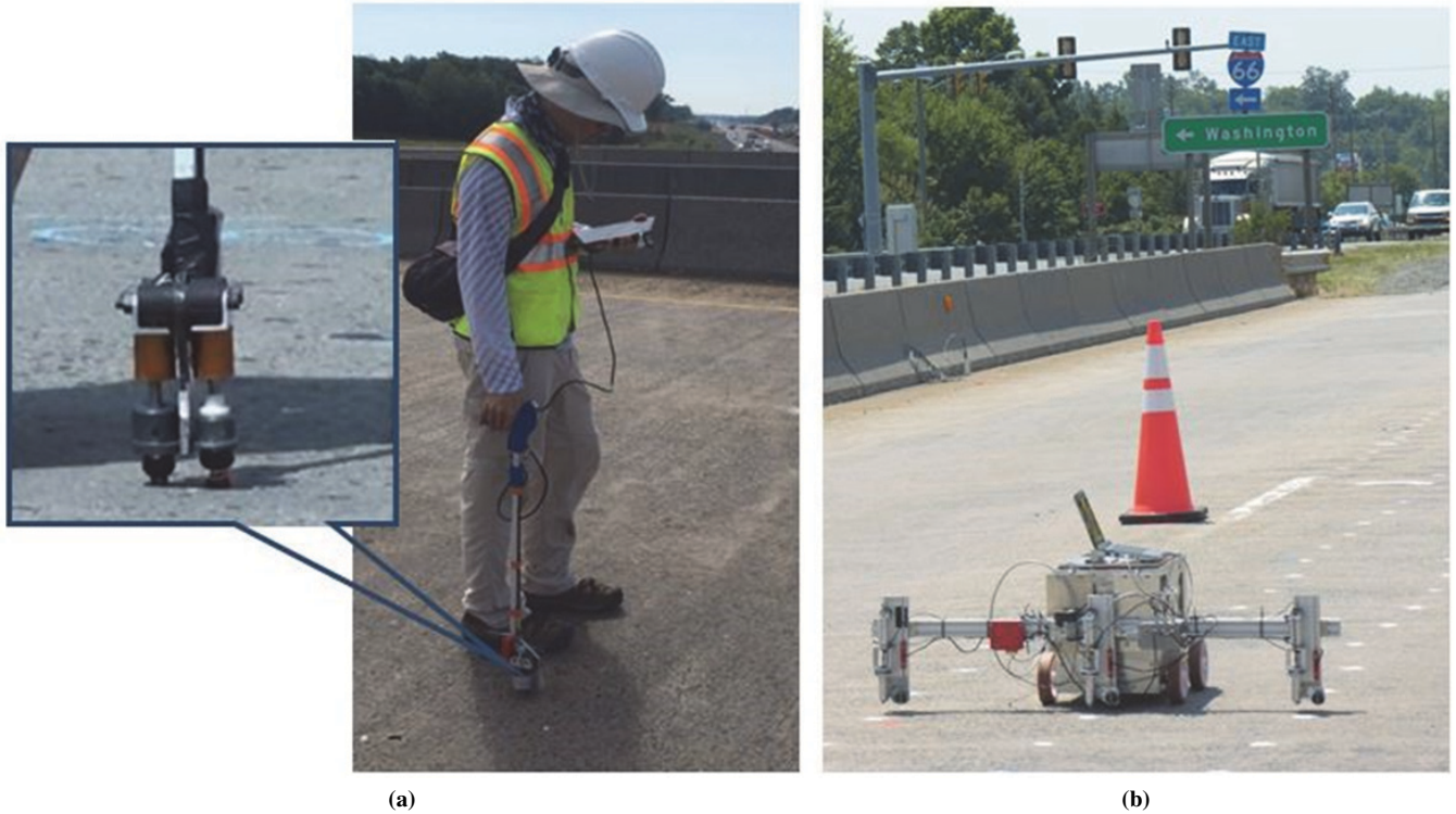
FIGURE 6 Two types of IE testing systems: (a) an IE cane and (b) a stepper.
