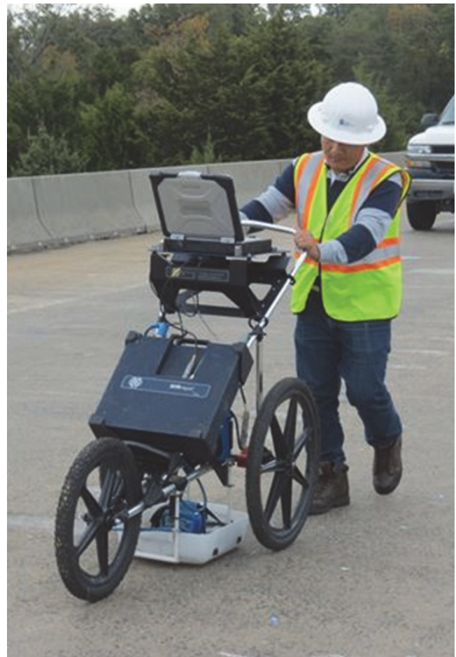
FIGURE 4 GPR survey using a 1.5 GHz ground coupled antenna.
