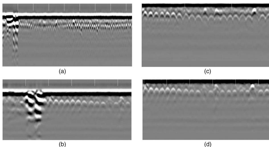
**Fig. 6.** (a) Unprocessed profile, 2008; (b) unprocessed profile, 2013; (c) processed profile, 2008; (d) processed profile, 2013
