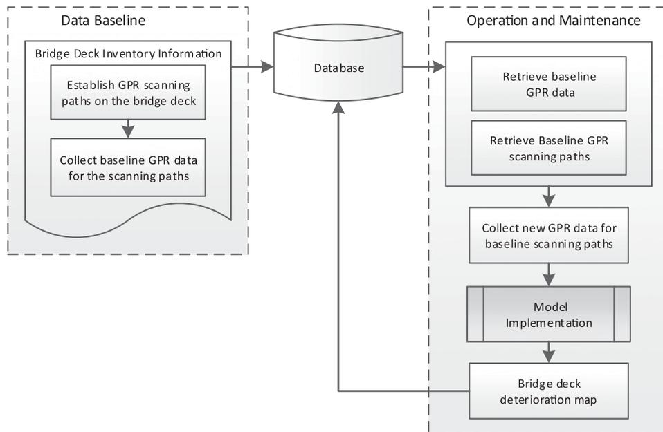
Fig. 4. Long-term condition assessment workflow of concrete bridge decks using GPR
