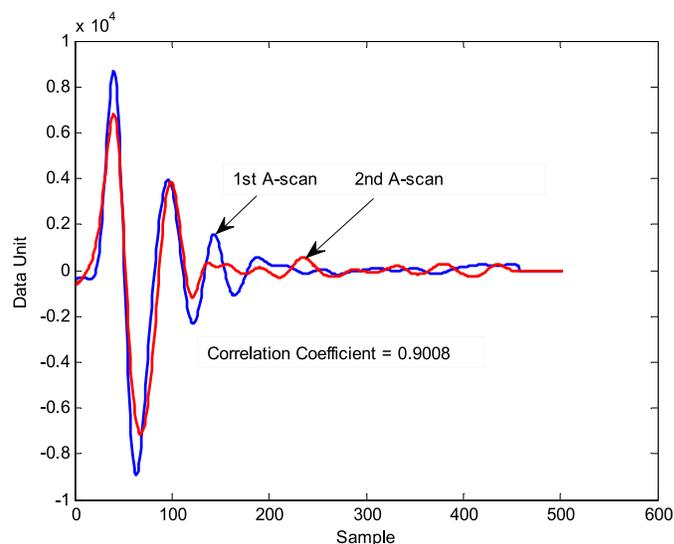
Fig. 5. Correlation between two GPR signals
