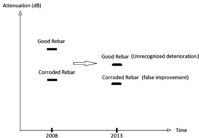
Fig. 8. Explanation for apparent deck improvement with amplitude interpretation
