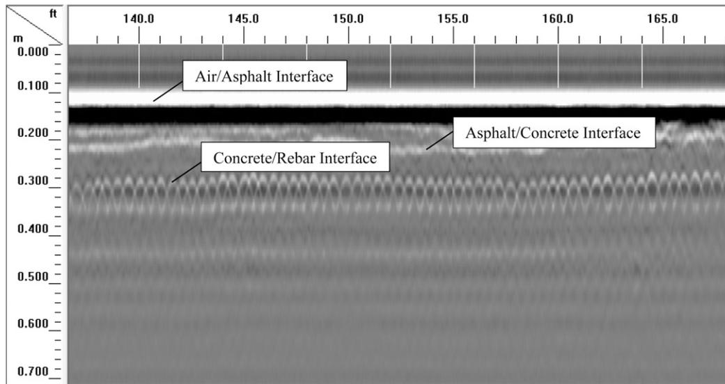
**Fig. 1.** Typical GPR image for concrete bridge decks with asphalt overlay
