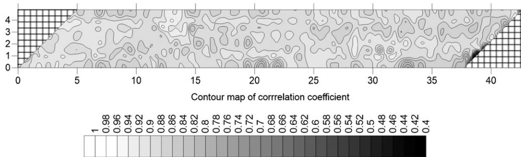
Fig. 7. Relative deterioration map between two consecutive scans
