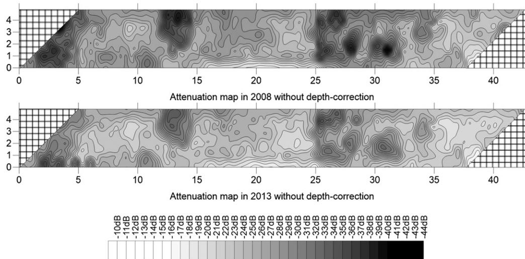
**Fig. 2.** Attenuation maps of two data sets without depth correction
