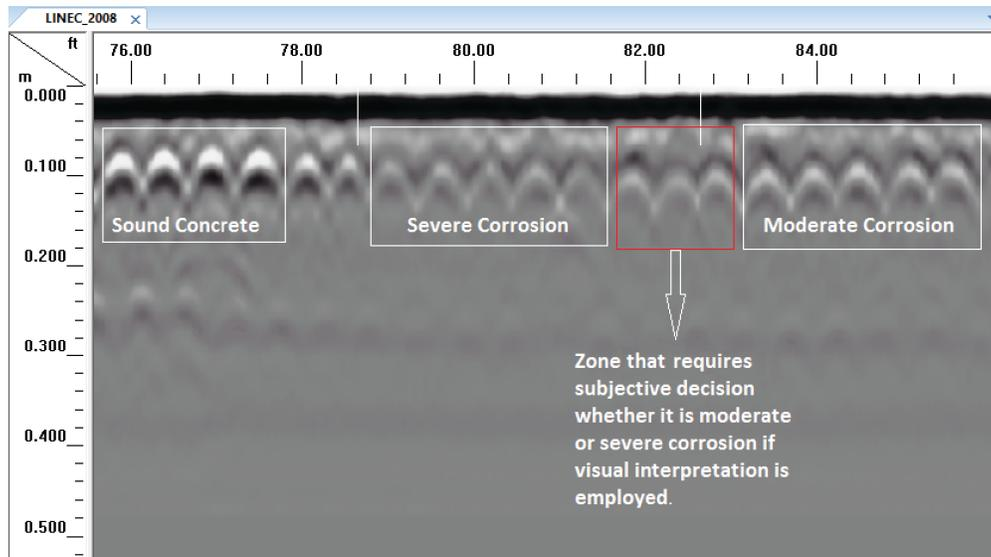
FIGURE 3 Visual examination of GPR profiles.
