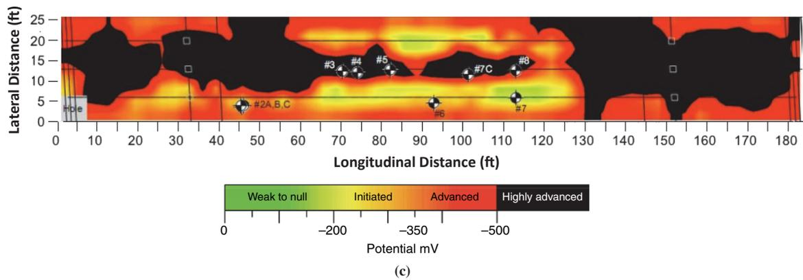
FIGURE 6 Condition maps provided by (a) proposed threshold model, (b) delamination testing, and (c) half-cell potential.
