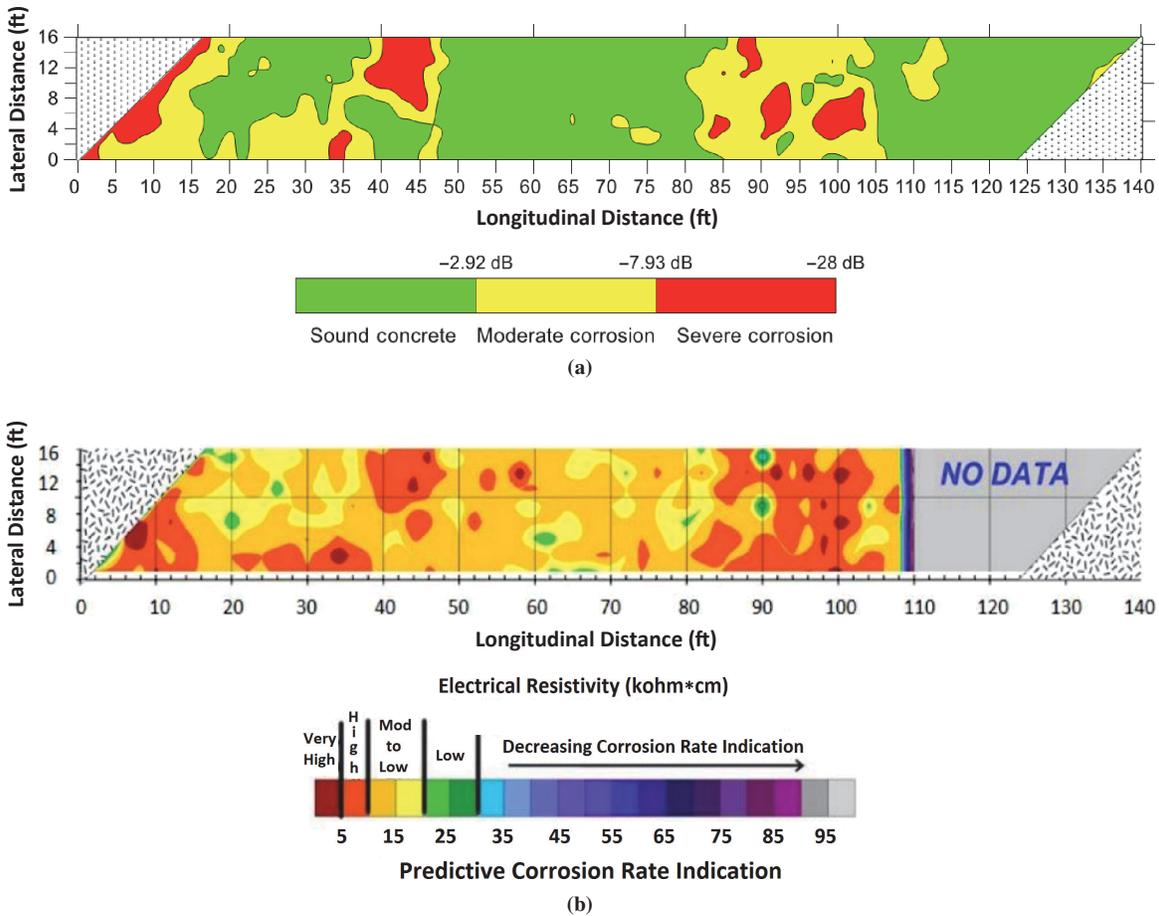
FIGURE 5 Corrosion maps based on (a) proposed threshold model and (b) concrete resistivity.
